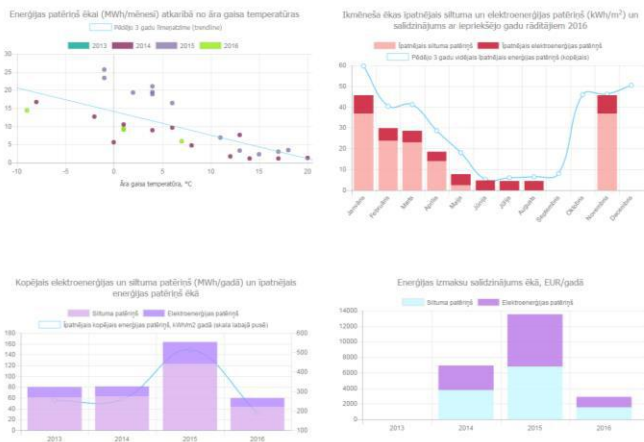
Example of analysis about a municipal building provided in the Online Energy Monitoring Platform
